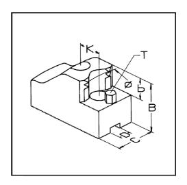
TuffGrip Hard Jaws are highly suited for aggressive gripping of 1<sup>st</sup> OP work and generally on black bar, castings or forgings. They provide secure grip and torque transmission
