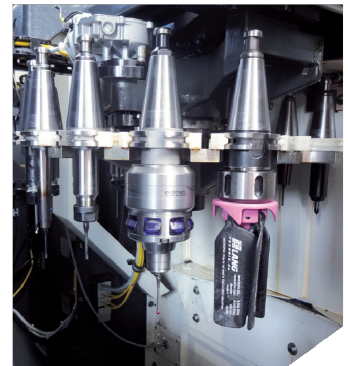
Clean-Tec is stored just like a common tool in the tool magazine and selected automatically via CNC programme.
