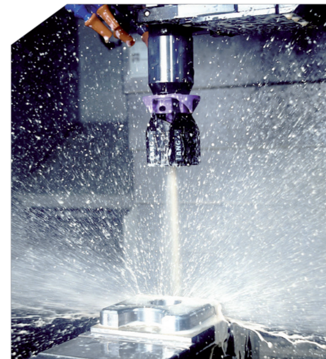
Workpieces and fixtures can be cleaned with coolant using the supply through the spindle.
