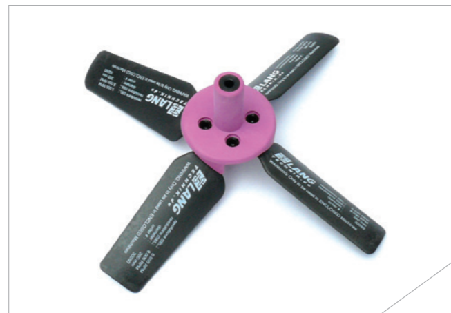
The Clean-Tec wings unfold and close automatically by switching the machine tool spindle on and off.
