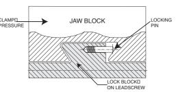
Quick Lock Jaw System – Jaws clip on to the lock block and are held by clamping pressure. Jaws are simply released by pushing in locking pin and lifting jaw away when clear of lock block.
