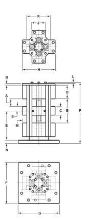
Included adapter plate fits Bock grid pattern, 80mm & 100mm machine pallets.
