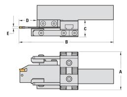
Please note dimension D (maximum depth of cut). If a greater depth of cut is required, we suggest using a separate cut-off tool and only using the bar puller for the pulling operation.
