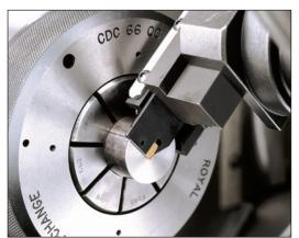
Cycle times are reduced because the turret does not need to index between cut-off and pulling operations.
