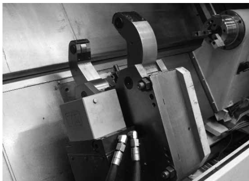
Example of power steady with side mount cylinder mounted to CNC Lathe
