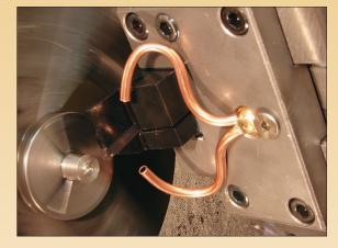
**TwinPop** nozzle shown installed in lathe turret.
