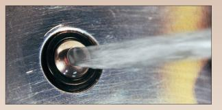
Simply insert the end of allen wrench (included) into the hole in the stainless ball until it engages the hex hole in the acetal body, then tighten the *PlugJet* into the tapped hole until the body is flush.
