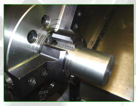
**Secure Pad Installation -** The ColletJaw System utilizes a dovetail anchor system to securely lock the pads in place, whilst feeding bar stock. This design places the bar thrust on the shoulder of the pad. There is no pressure on the clamp assembly because it is ideally positioned between the pad shoulder and the recess of the collet. The Pads cannot dislodge under normal use.
