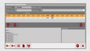
■ Data output in a format appropriate for the tooling machine controller (DOP), including format generator to generate post-processors / output formats (over 100 output formats are included in the EZset DOP library)
