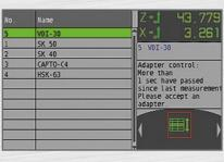
■ EZset zero point monitoring for 100% precise measurements after every adapter exchange
