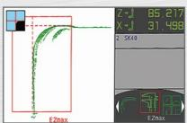
■ EZmax software function to determine and measure the maximum contour of
